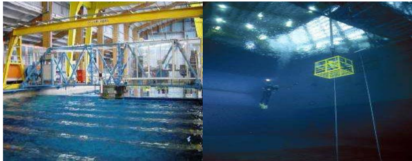
Wave basin with a wave energy converter under testing
